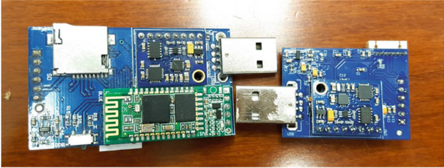
Fig. 4.4 Second generation IMU board. This module (right) consists in a combination of an IMU, a Bluetooth transceiver, a USB port (for power only). The earlier prototype version is shown on the left for comparison
