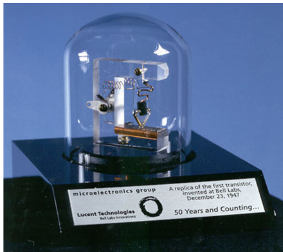
Fig. 1.2 Replica of transistor. Courtesy of Lucent Bell Labs
