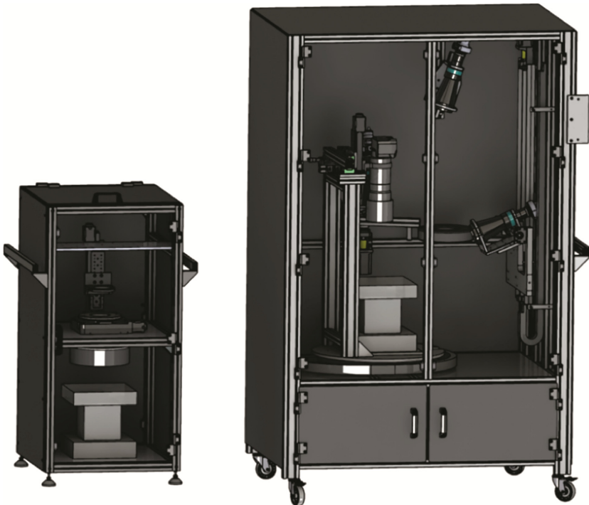
Fig. 1. View of two generations of PS equipment developed in ITAM. The height of the bigger one is approximately 170 cm. The object is placed on a table, where it is illuminated from different directions and inclinations by means of telecentric lamps (i.e. lamps whose beams do not broaden with distance, do not create a cone) and individual scenes are captured by a digital SLR camera.
