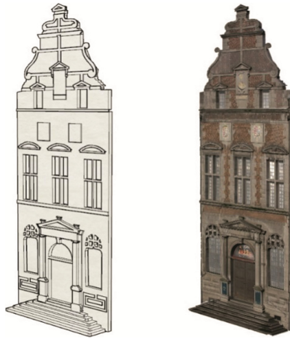
Fig. 1. Example of facade modelled with Rhino 3D and textured with picture
