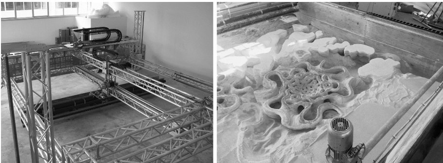
Fig. 4. Powder bed deposition 3D printer that allows the creation of free-form volumes. It consists of a sequence of nozzles that translate along the Cartesian area depositing sand and consequently the binder in all zones that are to be solidified. At the end of the process, the exceeding material is aspirated from the cavities in order to be reused (courtesy of Dshape ).
