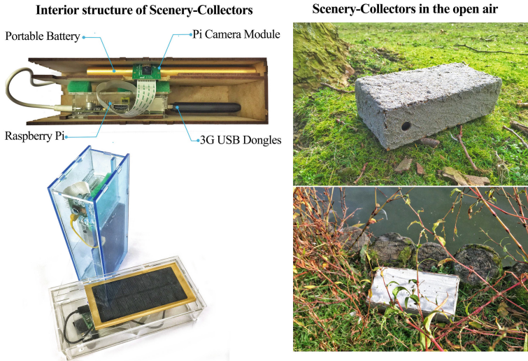
Fig. 5. Scenery-Collector and its interior structure
