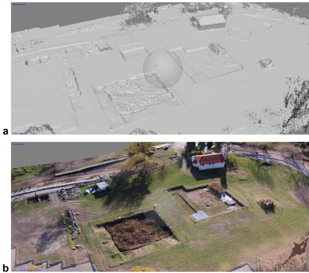
Fig. 12. a. Digital Surface Model (DSM). b. 3D photorealistic textured model of part of the archaeological site.
