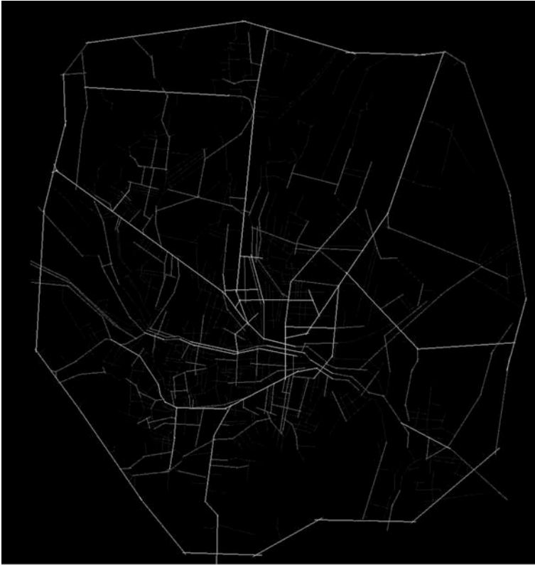
Fig. 4 Choice-to-depth map of Fayoum (white indicates high choice-to-depth value). Choice measures how likely an axial line or a street segment is to be passed through on all shortest routes from all spaces to all other spaces in the entire system (Hillier et al. 1987) Source Generated by DepthMap software
