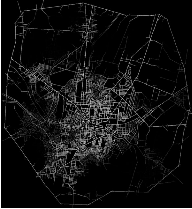
Fig. 3 Integration map of Fayoum (white lines indicate routes with high integration value). Integration is a normalized measure of distance from any a space of origin to all others in a system. It calculates how close the origin space is to all other spaces (Hillier et al. 1987) Source Generated by DepthMap software
