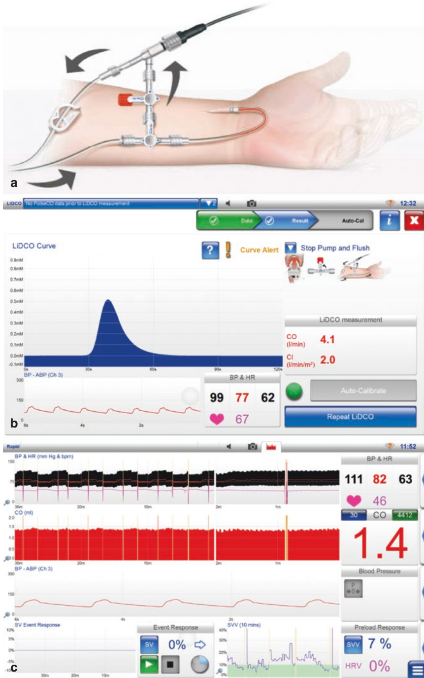
Fig. 5.9 (a) LiDCO ® lithium sensor attached to the patient; (b) LiDCOPlus ® system; (c) LiDCORapid ® system. With kind permission from LiDCO ® Ltd. London, UK
