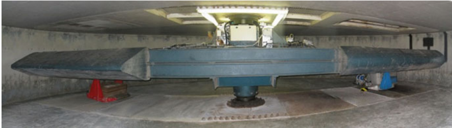
Fig. 16.1 A view of the 10 m diameter Turner Beam Centrifuge at University of Cambridge
