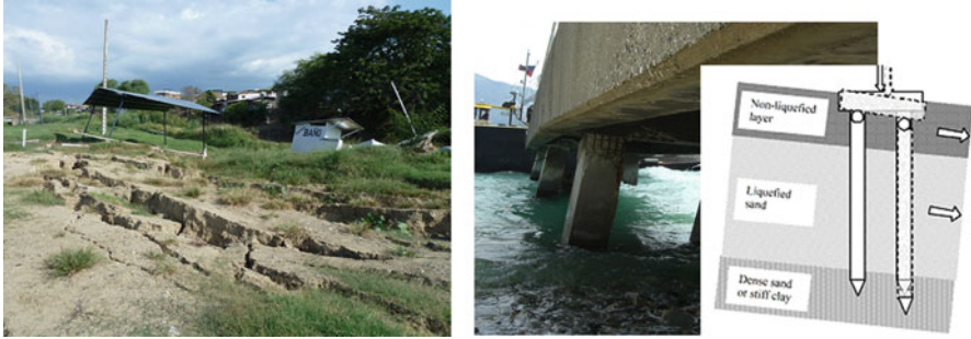
Fig. 16.11 Lateral spreading due to soil liquefaction and damage to pile foundations
