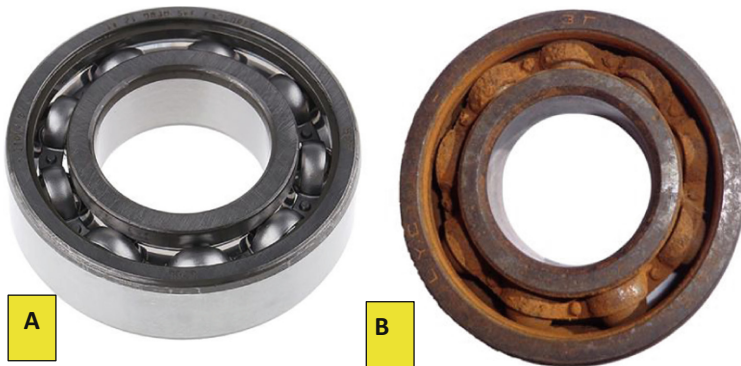
Fig. 2. The 6205 deep groove ball bearing used for the series of experiments. (A) new good bearing, (B) the corrosion-damaged gearbox bearing.
