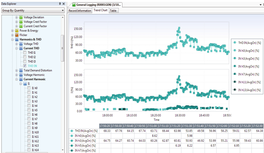
Fig. 2. Variation of current harmonics [%] of order 3, 5, 7, 11, 13 and of the total harmonic distortion factor [%], on the neutral conductor, within the time interval considered.
