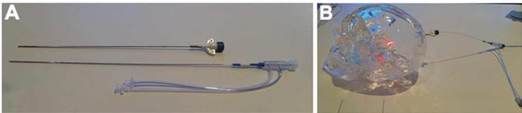
Fig. 19.2 (a) laser cooling catheter and stylets; (b) simulation of laser ablation amygdalo-hippocampectomy
