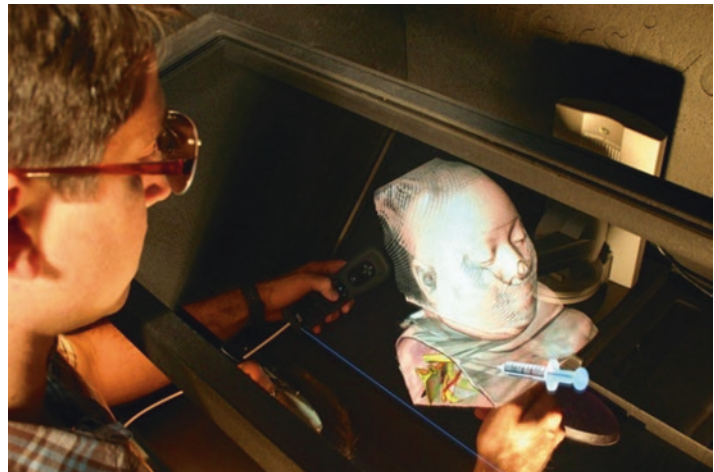
Fig. 11.16 Bimanual haptic simulator for medical training. (Courtesy of Ullrich et al. [14], used with permission)
