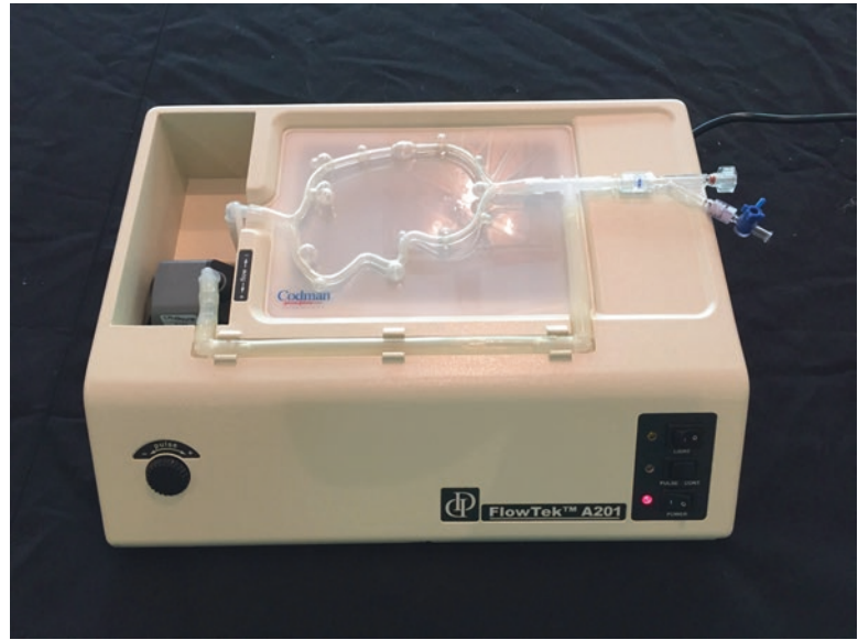
Fig. 6.2 A silicone flow model device with saline pump and simulated aneurysms
