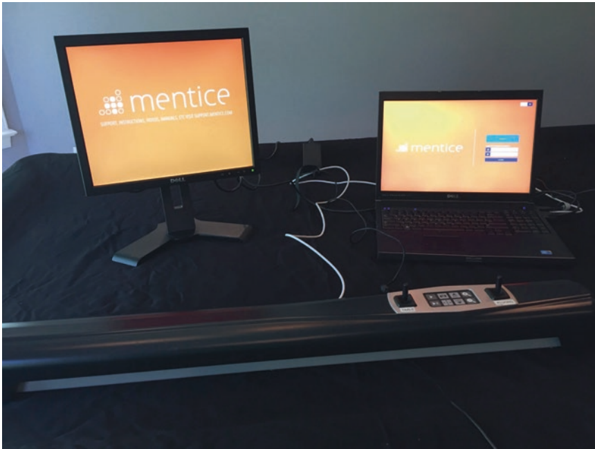
Fig. 6.3 The Mentice simulator with simulated table and foot pedal controls (not shown)
