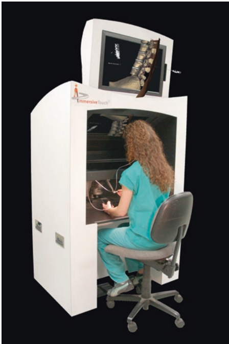
Fig. 18.1 The immersive simulation device. Seen are the box that contains the screen and robotic arms, as well as the foot pedal controllers, a 3D screen on top for additional viewers (Used with permission of ImmersiveTouch)
