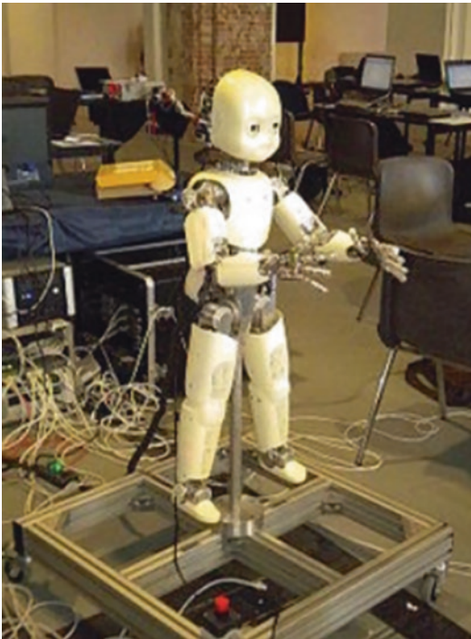
Fig. 22.2 An iCub robot mounted on a supporting frame. It was designed by the Robot Cub Consortium of several European universities and built by Italian Institute of Technology [56]
