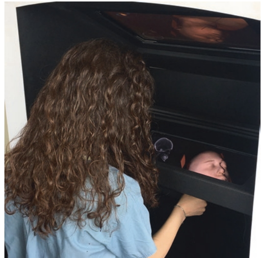
Fig. 14.2 ImmersiveTouch platform setup. The trainee looks into the screen that creates three-plane CT reconstruction (different modules available) wearing stereoscopic goggles that track head positioning and adjust virtual reality scene to viewer’s perspective. The non-dominant hand controls the SpaceGrip that allows the model positioning adjustment, and the dominant hand holds the haptic stylus that simulates the surgical tool (Used with permission of ImmersiveTouch)
