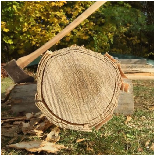
Fig. 4 When pounded, brown ash wood splits at the grown rings (photo by Suzanne Greenlaw)
