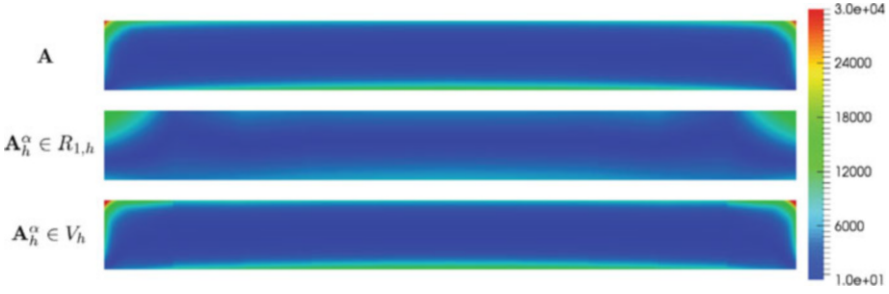
Fig. 12.2 Current distribution |j| = |\omega\sigma\mathbf{A}^\alpha| in plate plotted over cross-section y = 0 for \sigma_{\text{plate}} = 5 \cdot 10^7 , \delta_{\text{plate}}/h = 0.063
