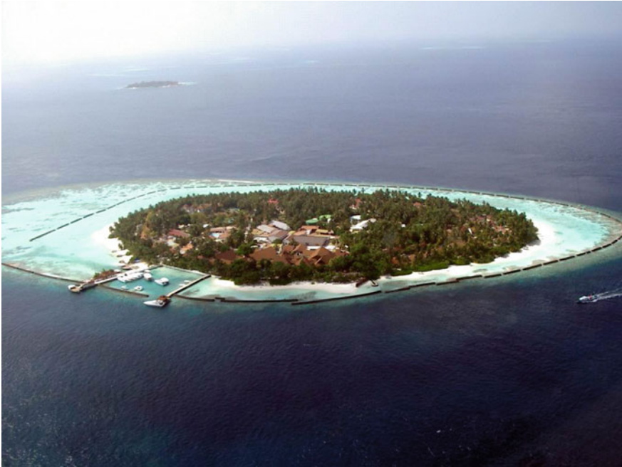
Fig. 5.13 A relatively narrow fringing reef, and a surrounding artificial berm, provide the only protection from the sea for the small island community on Kurumba Island, Maldives
