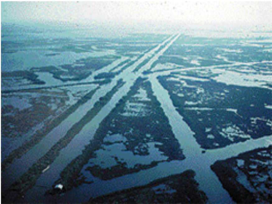
Fig. 13.7 Dredged access channels in Louisiana coastal wetlands. Photo source U.S. geological survey Louisiana coastal wetlands: a resource at risk. https://pubs.usgs.gov/fs/la-wetlands/
