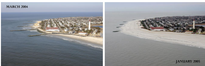
Fig. 11.5 Beach replenishment on the state park beach and around Cape May Point, before (left) and after (right) the restoration. Source U.S. Army Corps of Engineers 2007
