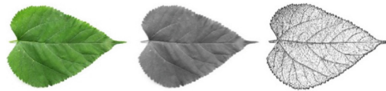
Fig. 5. Illustrated image with adaptive local threshold to mean (10), C = 0.2
