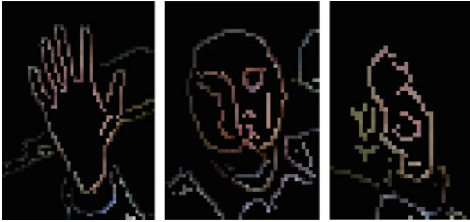
Fig. 3 The results of the edge detection (using Canny method) for each blob
