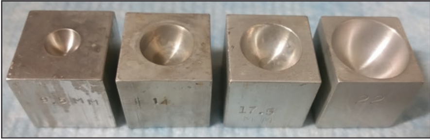
Fig. 72.2 Eyecup holders. Custom-made aluminum supports of different diameters (indicated on the sides) to fit eyes of various sizes. The supports are sterilized by autoclaving before use
