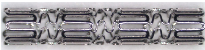
Fig. 18.2 Brightfield microscopy image of drug eluting stent (8 mm long Cordis Cypher ® stent)
