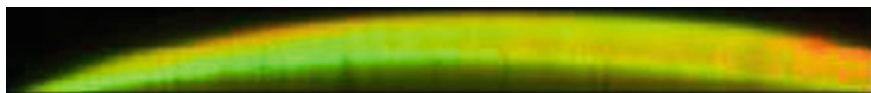
Fig. 18.9 Raman microscopic cross-sectional image of coating of 33 wt% dexamethasone in poly(butyl methacrylate) on stent. Red = Amorphous Dexamethasone, Green = Poly(butyl methacrylate). Image dimension = 100 \times 10 \mu\text{m}
