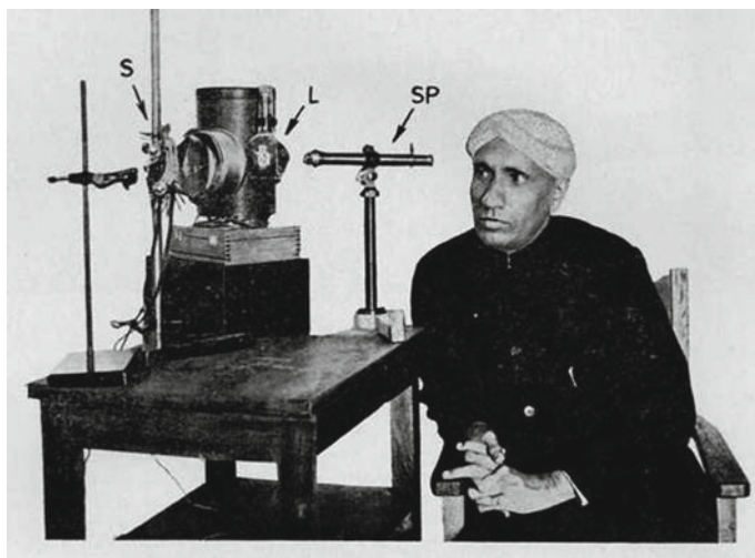
Fig. 1.8 Next step: Mercury lamp (S) and a simple hand spectroscope (SP) used for observing Raman spectra of liquid samples in large sample cells (L). Raman used his eye as the detector
