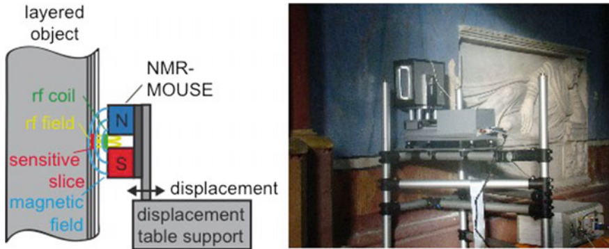
Fig. 2 The NMR-MOUSE. a Drawing of the sensor mounted on a displacement table for measuring depth profiles through vertical layer structures such as mortar layers covering walls. The radio-frequency (rf) coil transmits the excitation impulses and receives the signal. b Setup of the sensor measuring a depth profile of the natural moisture content through a painted, wet wall in the chapel of St. Mary in Chaalis
