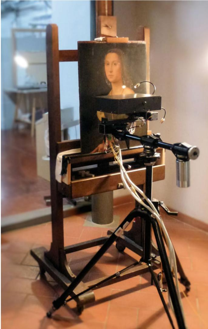
**Fig. 1** An in-situ examination of Raphael's *La Muta* in 2014 at Opificio delle Piere Dure in Florence, Italy with the portable OCT tomograph constructed at Nicolaus Copernicus University in Toruń
