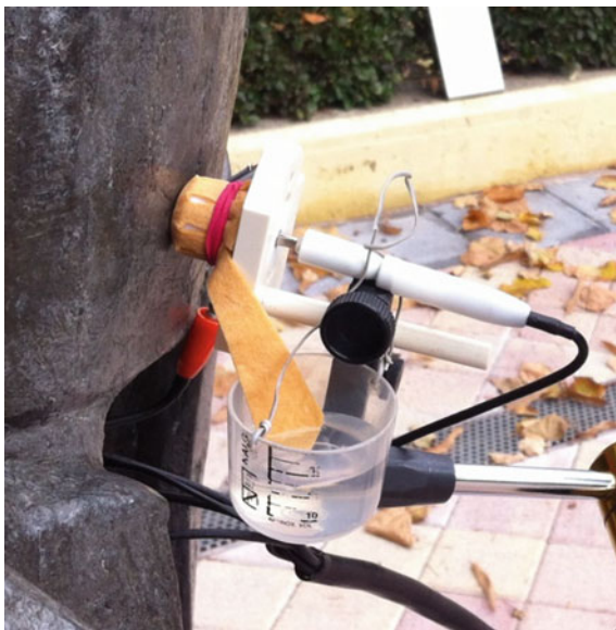
Fig. 5 Contact cell designed by P. Letardi
