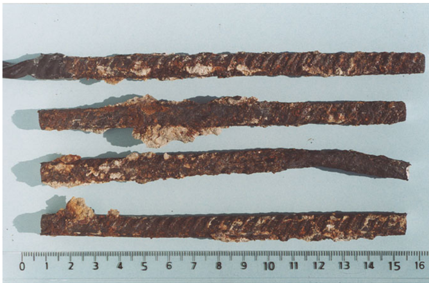
Fig. 12 Corroded rebars showing the oxide scale
