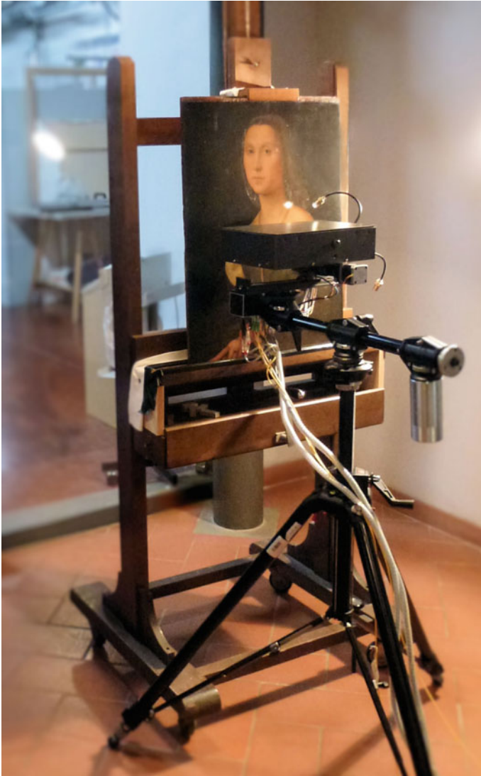
Fig. 1 An in-situ examination of Raphael's La Muta in 2014 at Opificio delle Piere Dure in Florence, Italy with the portable OCT tomograph constructed at Nicolaus Copernicus University in Toruń
