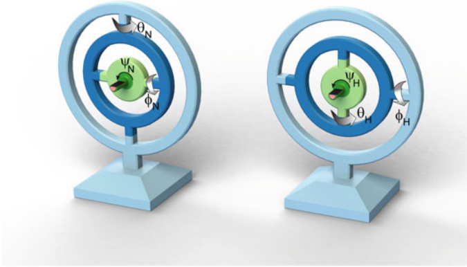
Fig. 3.11 In gimbal systems, the axes of rotation are determined by the geometry of system. Both gimbals in this figure are in the reference orientation. Let \mathbf{b}_x , \mathbf{b}_y , \mathbf{b}_z describe a body-fixed coordinate system. Left In a nautical (Fick) gimbal , the orientation of the object (the turn on the inner dial) is completely characterized by a rotation about the vertical axis \mathbf{b}_z by \theta_N , followed by a rotation about the (rotated) horizontal axis \mathbf{b}_y by \phi_N , and a rotation about the (twice-rotated) dial-axis \mathbf{b}_x by \psi_N . Right In a Helmholtz gimbal , the orientation of the inner dial is characterized by a rotation first about the horizontal axis \mathbf{b}_y by \phi_H , followed by a rotation about the (rotated) \mathbf{b}_z axis by \theta_H , and then a rotation about the dial-axis \mathbf{b}_x by \psi_H
