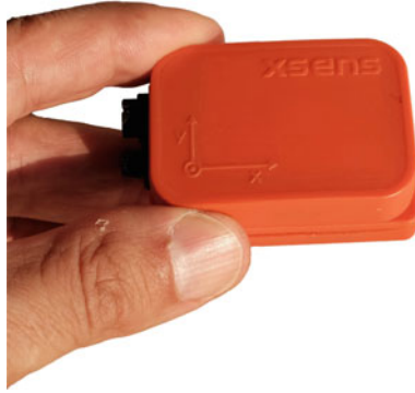
Fig. 2.6 The MTX sensor from Xsens measures linear acceleration, angular velocity, and the local magnetic field
