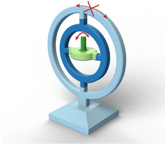
Fig. 3.14 Gimbal lock: the orientation of the innermost axis cannot be reoriented in the direction of the dotted arrows
