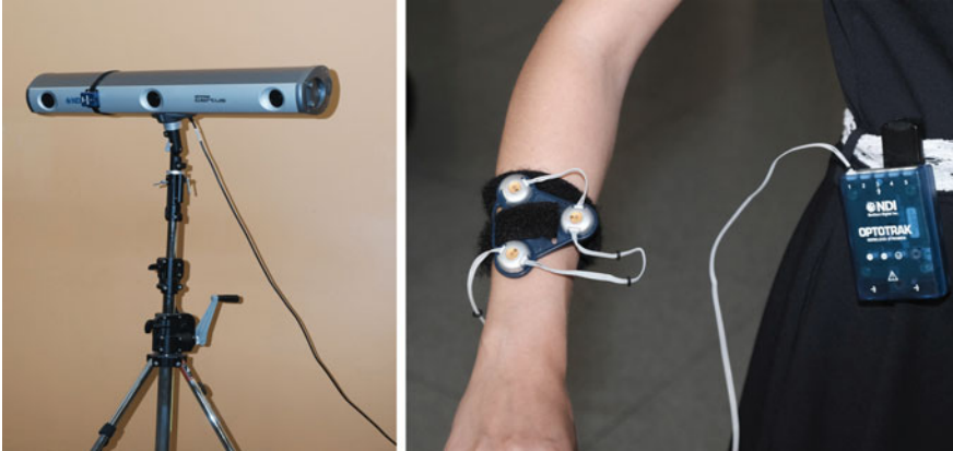
Fig. 2.2 Left: The Optotrak sensor with three cameras, mounted on a tripod. Right: The corresponding active markers (here three combined), with the communication unit to communicate with the sensors
