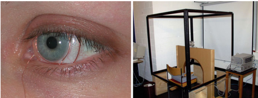
Fig. 2.17 Left: Scleral search coil from the company Skalar . Right: External magnetic field frame
