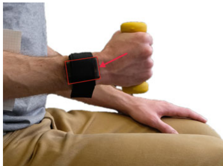
Fig. 2.5 Inertial sensor from x-io Technologies (red box/arrow) attached to the wrist during a physiotherapy exercise
