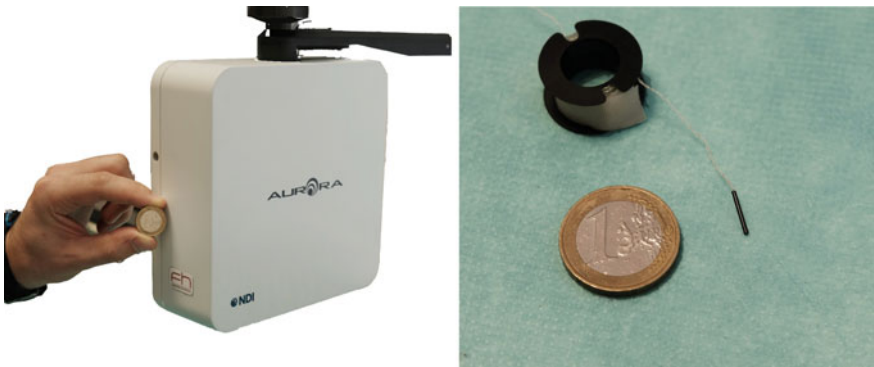
Fig. 2.19 Induction systems with inhomogeneous magnetic fields generated by a small magnetic field generator can determine not only the orientation of the sensor in space but also its position. Left: The Aurora system from NDI. Right: the corresponding, tiny sensor coils (inside the tubular black shielding cover)
