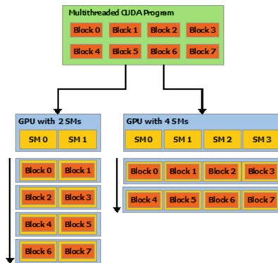
Fig. 1. From [6]: A multithreaded program is partitioned into blocks of threads that execute independently from each other, so that a GPU with more multiprocessors will automatically execute the program in less time than a GPU with fewer multiprocessors.
