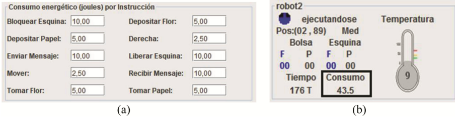
Fig. 2. ECMRE (a) Energy consumption by instruction in the Robot/Processor section, (b) Execution Information area, where robot energy consumption information is displayed
