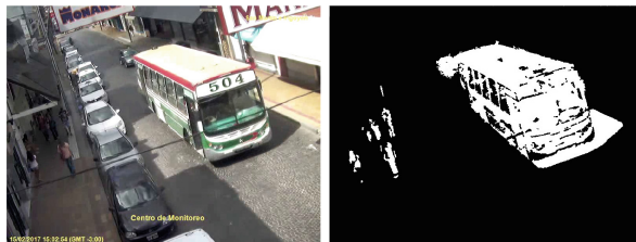
Fig. 2. Video image, left, and background subtraction with ViBE, right, for a video captured in a video surveillance camera.
