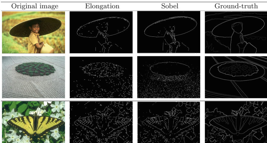
Fig. 4. Original images and output images, produced by the new method and by Sobel method, and ground-truth images are in the 1st, 2nd, 3rd, and 4th column, respectively.
