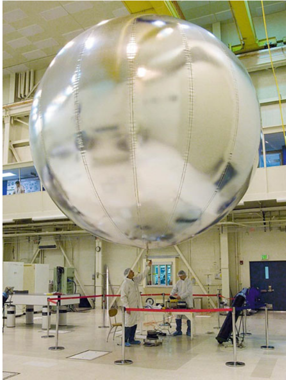
Fig. 4.23 Venus balloon prototype (5.5 m diameter, 4.5 kg payload capacity). The balloon includes an exterior Teflon film for protection from sulfuric acid in the Venus clouds
