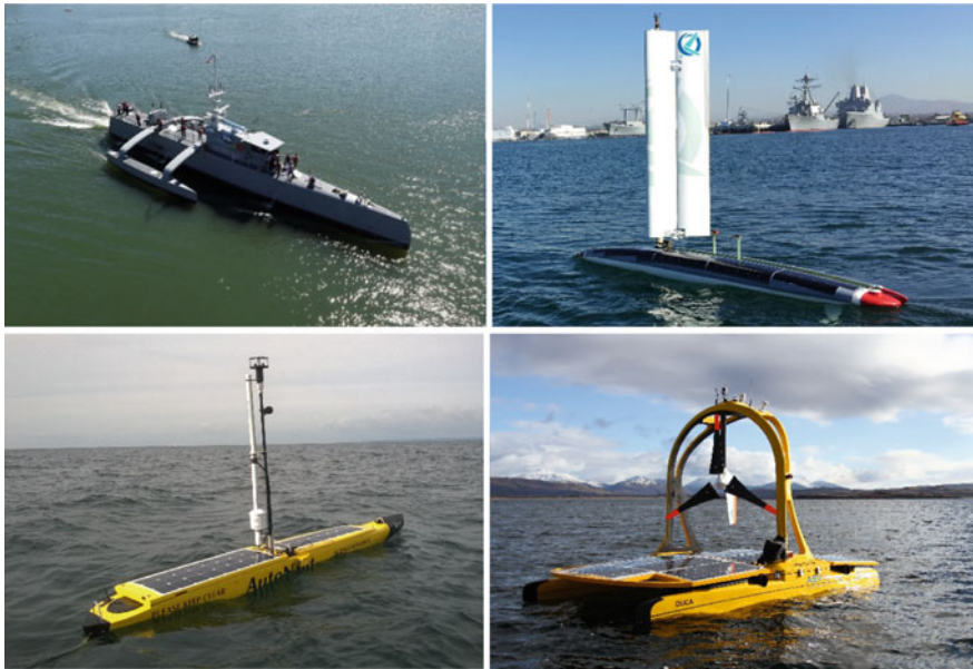
Fig. 5.3 Examples of Unmanned Surface Vehicles: DARPA’s Sea Hunter, (top left), Ocean Aero’s Submaran (top right, Copyright Ocean Aero Inc. Used with permission.), AutoNaut (bottom left, Copyright AutoNaut Ltd, with permission), ASV Global C-Enduro (bottom right, Copyright ASV Global, used with permission)
