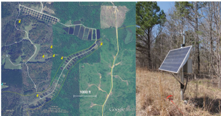
Fig. 3.17 Layout of the seven element array used in conjunction with the porous metal dome measurements
