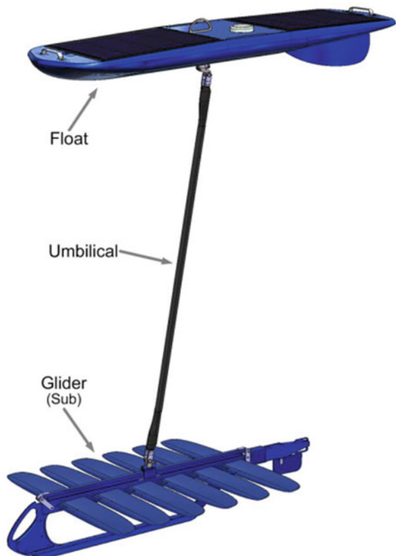
Fig. 5.21 The Wave Glider ® SV2—designed and manufactured by Liquid Robotics, Inc. Image used with permission
