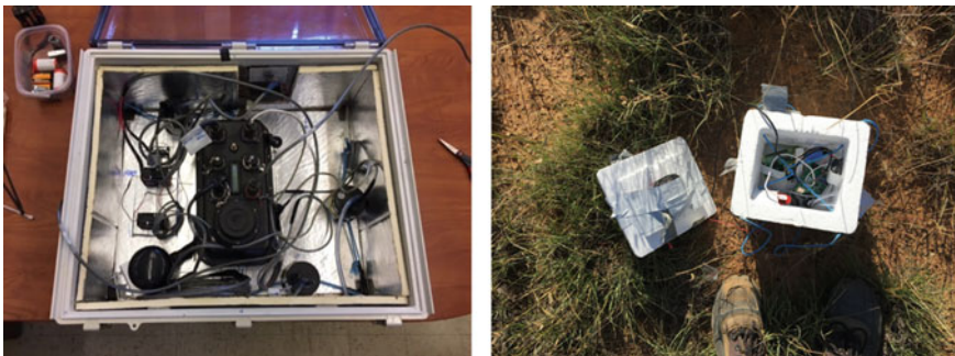
Fig. 4.9 An infrasound payload for the HASP 2016 flight (left). Note the hard-shelled box, inner layer of insulation, and secure equipment mounting. The entire enclosure was covered in white tape before flight. The SISE/USIE solar balloon payload box (right) was constructed from the inner lining of a medical-grade foam shipper. This photo was taken during recovery of the payload and envelope several weeks after landing. The box was opened prior to taking the photo
