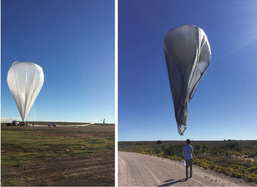
Fig. 4.4 A zero pressure balloon (left) and a solar hot air balloon (right) launched during the SISE/USIE infrasound experiment
