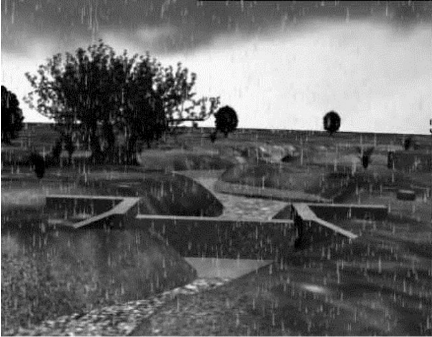
Fig. 18.8 Direct surface recharge through check dam
