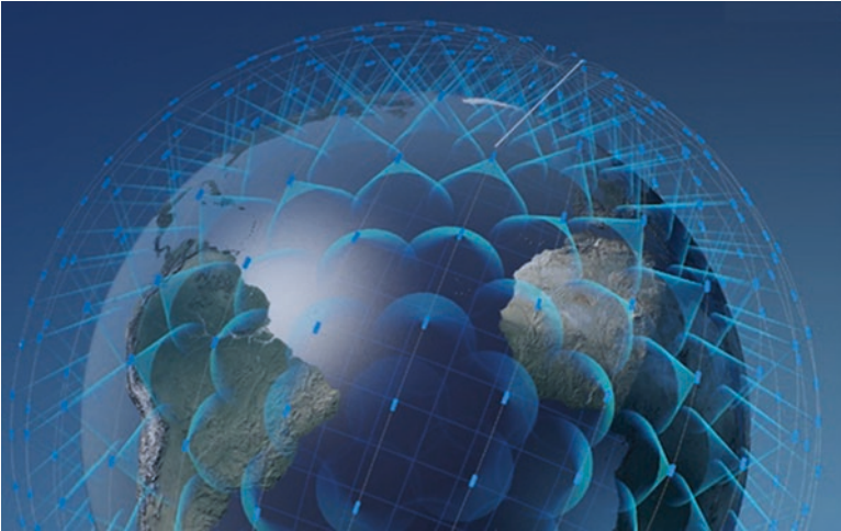
Fig. 7.3 The OneWeb megaLEO system that will involve nearly 1,000 smallsats orbiting in 800 to 950 km orbits. (Graphic courtesy of OneWeb)
