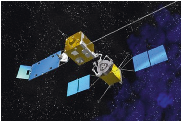
Fig. 6.2 MDA on-orbit servicing vehicle approaching to capture a satellite. (Graphic courtesy of MDA)
