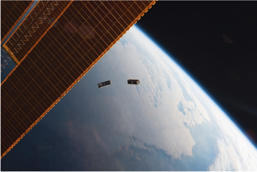
Fig. 5.2 Two of Planet's 3-unit Dove satellites shortly after deployment from the NanoRacks Cubesat Deployer on the International Space Station on May 17, 2016. (Image courtesy of NASA. Source: https://www.nasa.gov/image-feature/cubesats-deployed-from-the-international-space-station )
