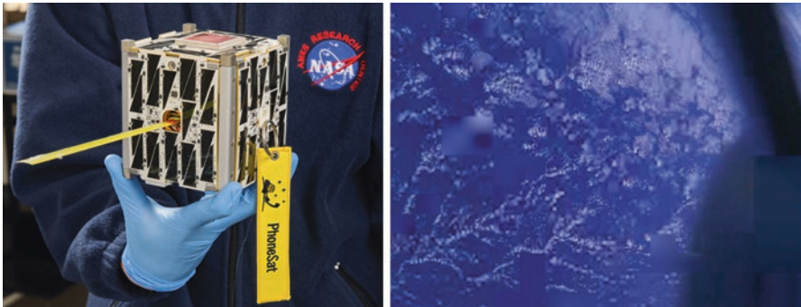
Fig. 3.6 The NASA Ames PhoneSat with antenna made from a yellow tape measure (left) and an image taken from space using the smartphone camera (right). (Graphics courtesy of NASA)
