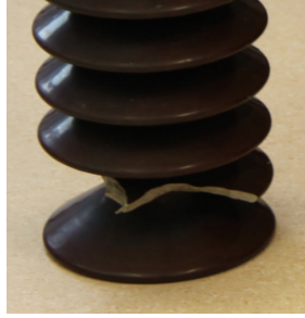
Fig. 2. Example of a porcelain long rod insulator (type LP 75/14/860) with a chipped disc.
