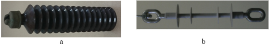
Fig. 1. Examples of electrical insulators: (a) Porcelain long rod line insulator (LP 75/14/860), (b) Composite string insulator (CS 70 E24 170/650).
