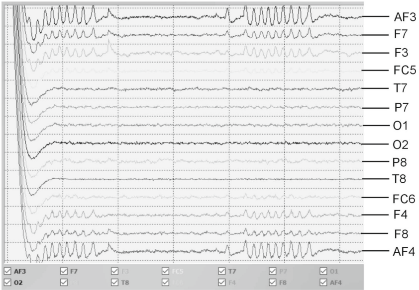
Fig. 2. EEG signal registered during simultaneous left and right eye blinking activity. EMOTIV brand 14 electrode EEG helmet.
