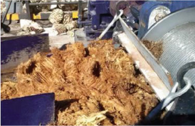
Fig. 3 Residual fiber, commonly known as bagasse, after agave juice extraction, Rudio Distiller, Jalisco, Mexico
