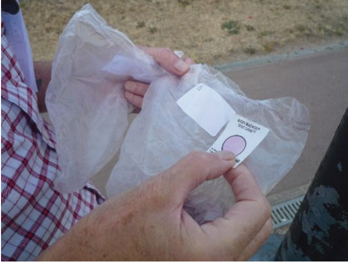
Fig. 27.2 Testing Eco-Badge ozone detection kits on the Pepys Estate
