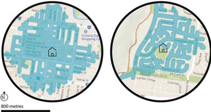
Fig. 18.2 Radial buffer (circle) and road network buffer (shaded) on grid-patterned street network (left) and curvilinear-patterned street network (right)
