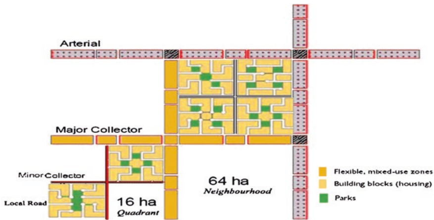
Fig. 19.4 (a) Neighbourhood road network patterns (Wei and Lovegrove 2012). (b) Neighbourhood road network patterns (Wei and Lovegrove 2012)
