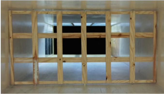
Fig. 4 Uniform grid with 6 \times 3 cells
