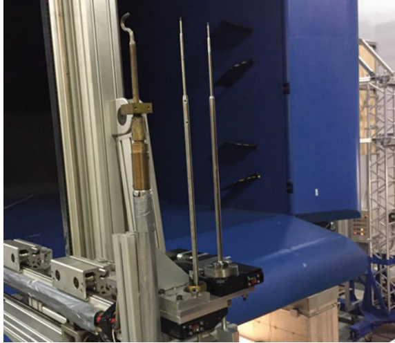
Fig. 4 Probe system mounted on the traversing in 2016 test campaign
