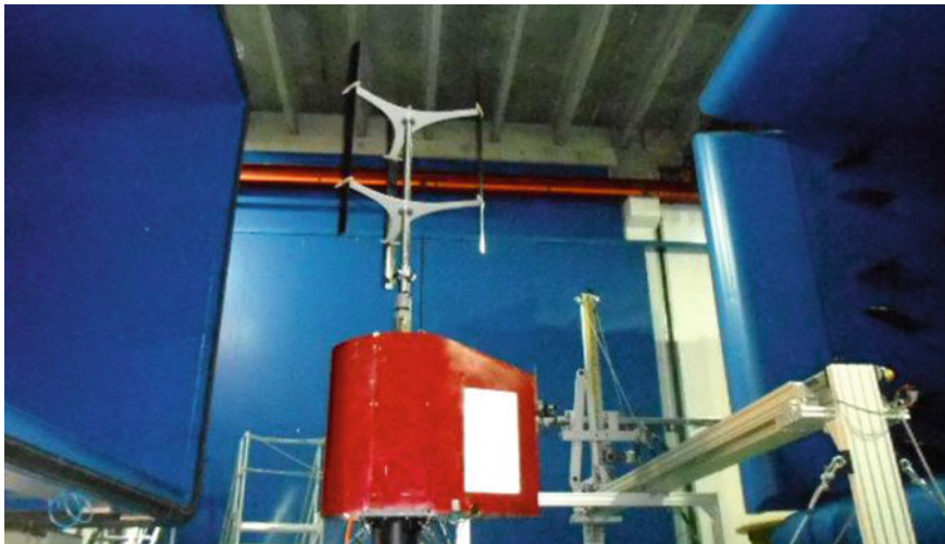
Fig. 2 Side view of the test section with the H-shaped rotor and the traversing system (on the right)
