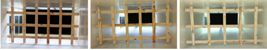
Fig. 6 Different modifications of the grid to obtain uniform flow. From left to right, grids 2 ( M = 0.33 m), 3 ( M = 0.35 m) and 4 ( M = 0.40 m)
