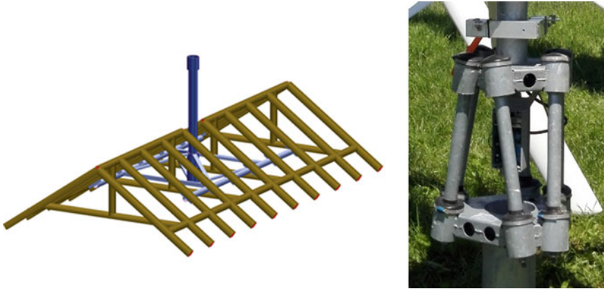
Fig. 5 Mast junction with the gabled roof (left) and oscillation decoupler for VASWT (right)
