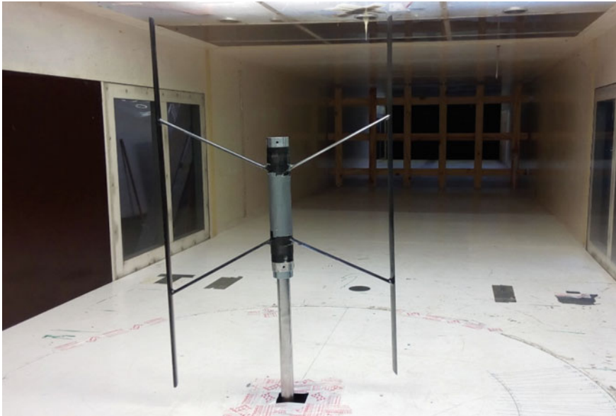
Fig. 9 VAWT turbine placed in the wind tunnel, with the turbulence grid 3.75 m upstream
