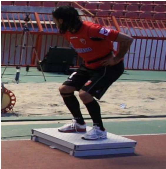
Fig. 1. Performing of the jumping on the force plate platform
