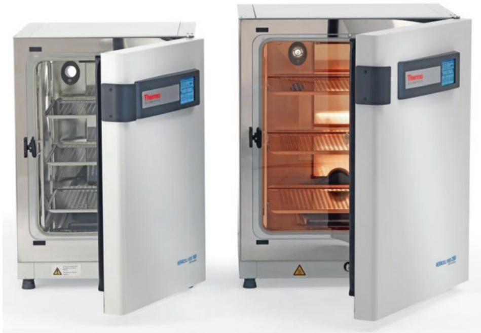
■ Fig. 2.6 Incubators for mammalian cell cultures (Thermo Scientific Laboratory Products, Germany)
