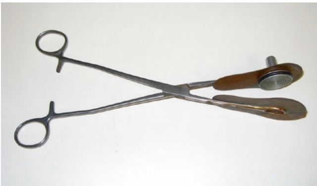
Fig. 2.3 Modified obstetric clamps, shown with mounting disc inserted
