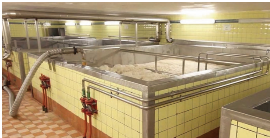
Fig. 11.3 Square tank for wheat beer fermentation
