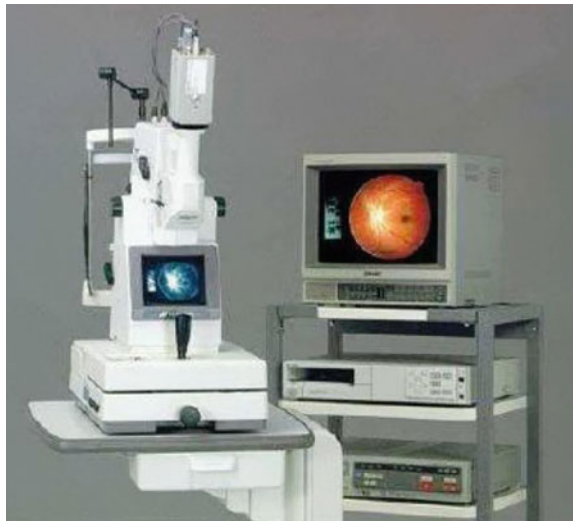
Fig. 2 A fundus camera and its accessories
