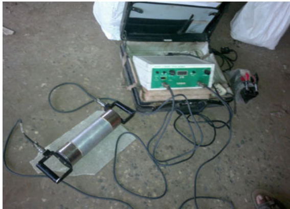
Fig. 3 Ultrasonic pulse velocity meter being calibrated before testing
