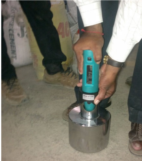
Fig. 2 Digital silver schmidt rebound hammer being calibrated on the standard Anvil
