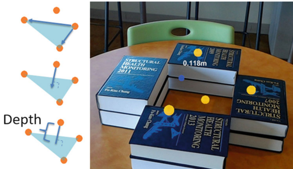
Fig. 23.5 An illustration of how depth is calculated along with what the user would see when the app is in use
