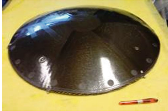
Fig. 13.2 DUT: Antenna reflector kindly provided by Thales Alenia Space
