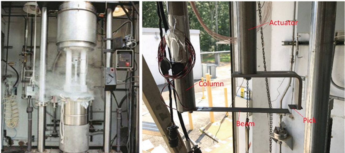
Fig. 34.4 Cryostat and cantilever beam test setup
