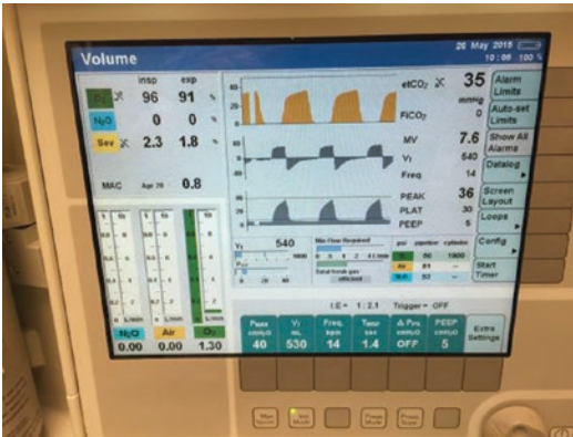
Fig. 81.2 Classic respiratory pattern observed in obese patients: increased peak pressures, obstructive pattern, and absence of plateau
