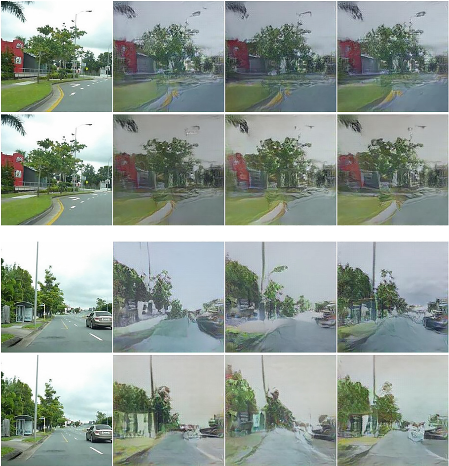
Fig. 6. Test sample (first column) and images synthesized to yield the same descriptor as the test sample. Caffenet (conv5) is shown on top, and Hybridnet (conv5) on the bottom.
