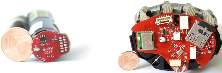
Fig. 1. Prototype implementation of the new electronics for the hand prosthesis. Each of the four main digits (index, middle, ring and small finger) has its own motor control board (left) which offloads movement tasks from the main processor (right). The latter controls the motor for the thumb (not shown) and interfaces the peripherals, such as the Bluetooth module and SDcard shown in the right image.
